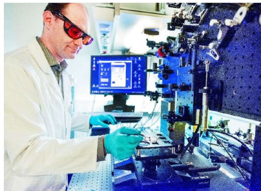
Image of the current maskless laser lithography setup at Joanneum Research MATERIALS
