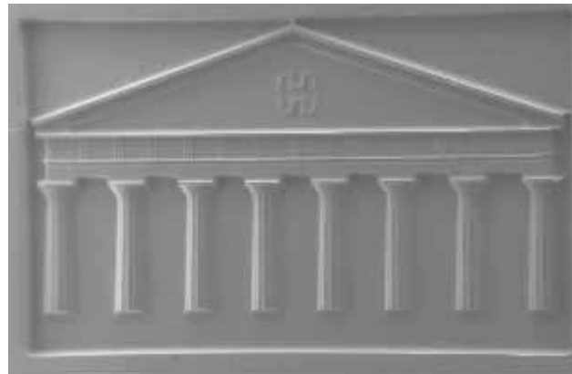
Temple, 120 µm deep, FT~180 µm (double coat; 10 mm writing head, CI-Over 40, 2 h develop)
