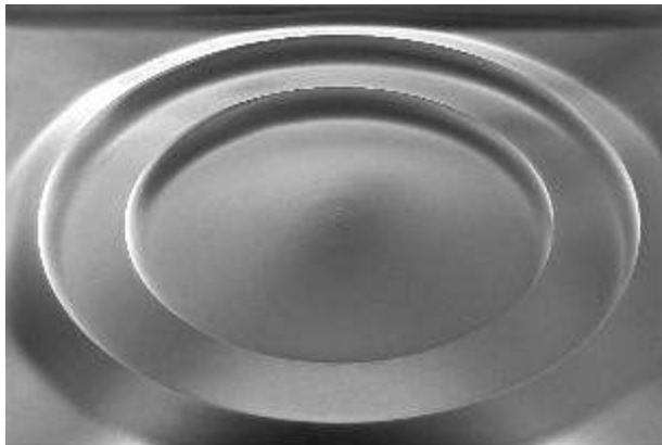
Fresnel lens, 103 µm deep, 2 mm \varnothing , FT~120 µm (single coat; 4 mm writing head, CI-Over 20, 1.5 h develop)
